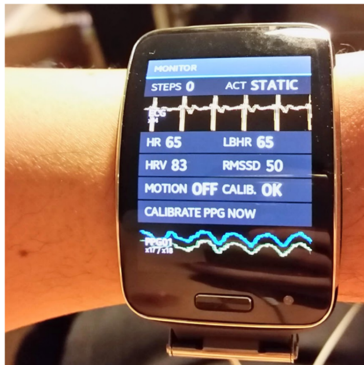
Figure 1. Samsung Simband 2 smartwatch showing simultaneous single-lead ECG (electrocardiogram) and PPG (photoplethysmogram) recordings.
