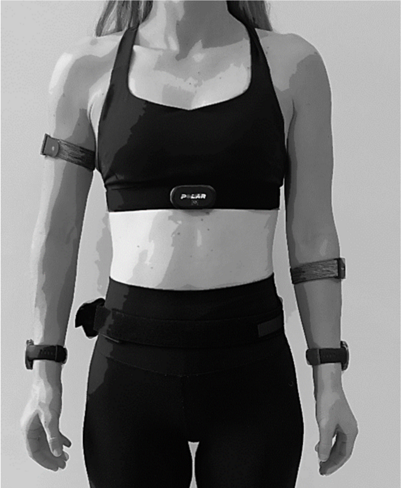
Figure 2. Placement of the different wearable devices. The H10 chest belt was placed on the chest with a Vantage V2 as logger on the waist. A Vantage V2 was placed on each wrist. A Verity Sense was placed on the upper arm and forearm.
