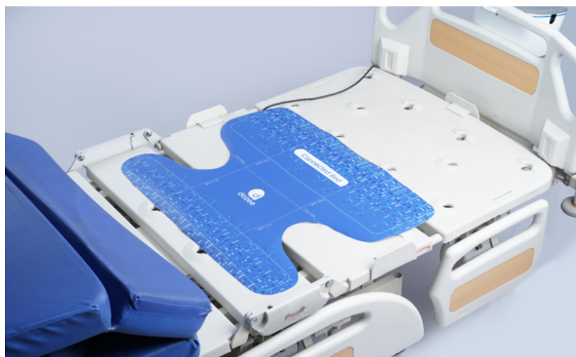
Figure 1. A sensor sheet positioned beneath the bed captures subtle microvibrations from the patient, enabling noninvasive measurement of vital signs.
